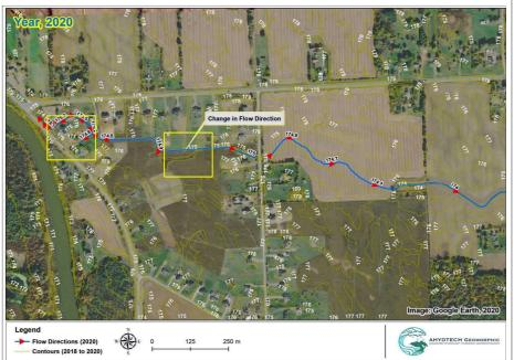
2020 shows the flow direction location change location like 2018. In the West channel, a 0.6m diameter and 125m long culvert runs in between 275 Victoria Avenue and 285 Victoria Avenue properties which runs 35m in between the two properties and then turns 90 degrees under the ditch along Victoria Avenue and the West Channel downstream.
