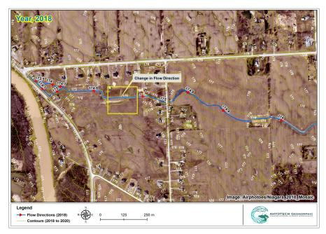
2018 shows the change in flow direction location shifted towards the west of Farr Road. Development through residential houses took place within the area compared to 2010. An additional channel is seen between two properties at the Victoria Avenue properties which turns at an angle of 90 degree (approx.)
