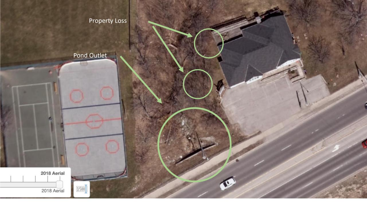
Close up of the stormwater pond outlet at Hwy20 showing erosion of the bank below the Pelham Cares building.
