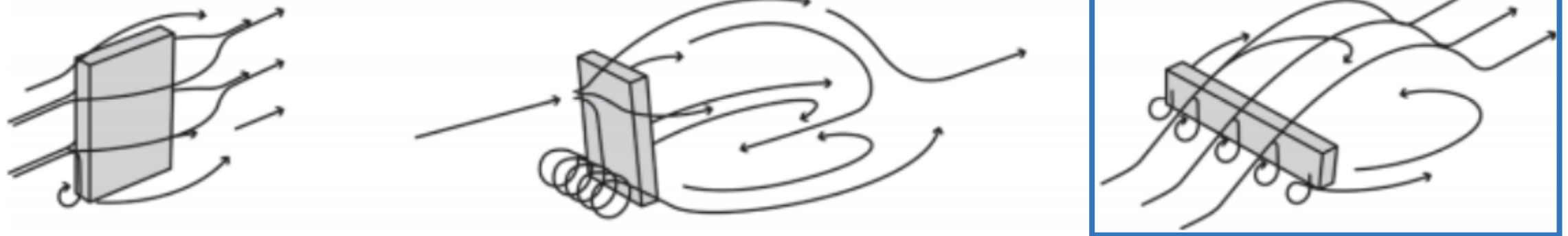
Figure 1: Airflow around a tall and slender building, a tall and wide building and a low and wide building.
