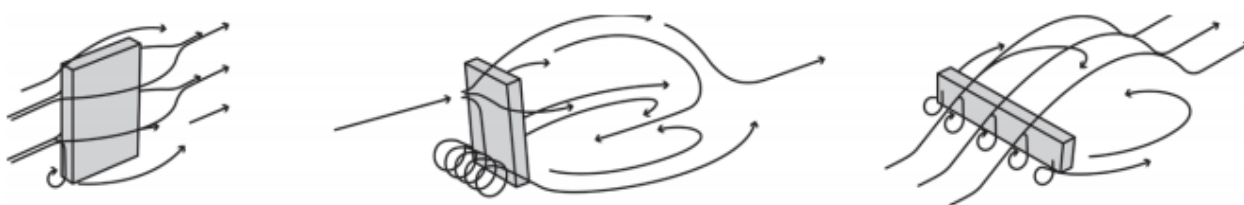
Figure 1: Airflow around a tall and slender building, a tall and wide building and a low and wide building. Image Source: Pijpers-van Esch, Marjolein. (2015). Designing the Urban Microclimate. A framework for a design-decision support tool for the dissemination of knowledge on the urban microclimate to the urban design process. A+BE: Architecture and the Built Environment.
