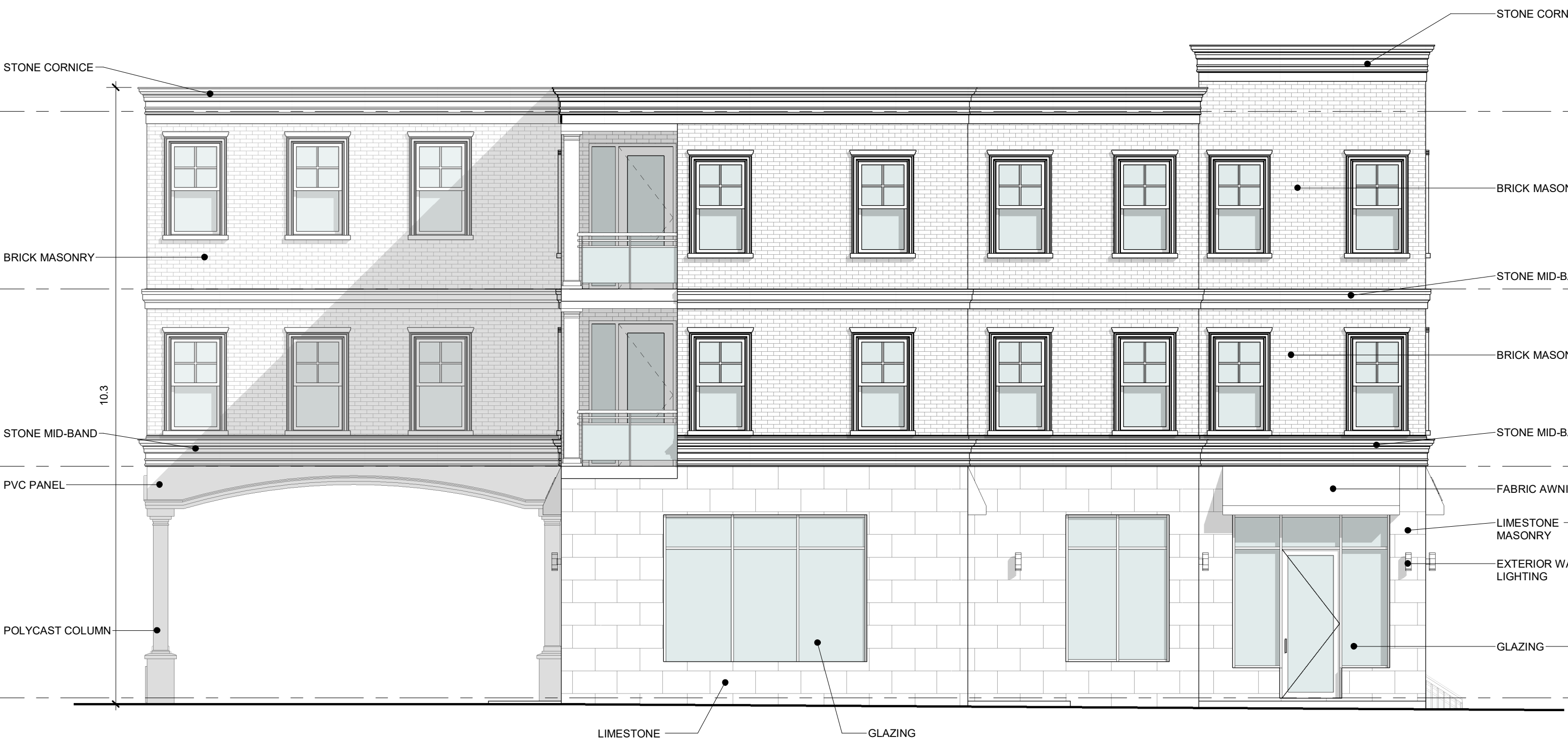
⑥ NORTHEAST ELEVATION 3/16" = 1'-0"
